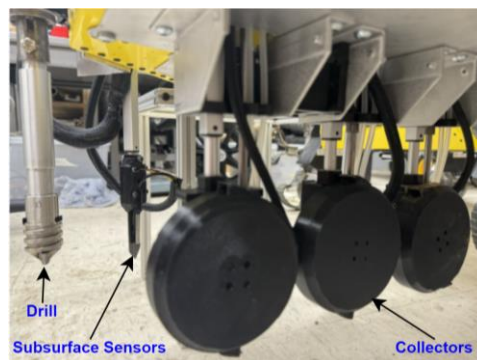
Figure 1: External View of Science Package
