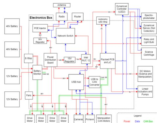
Figure 3: Electronics System Diagram
