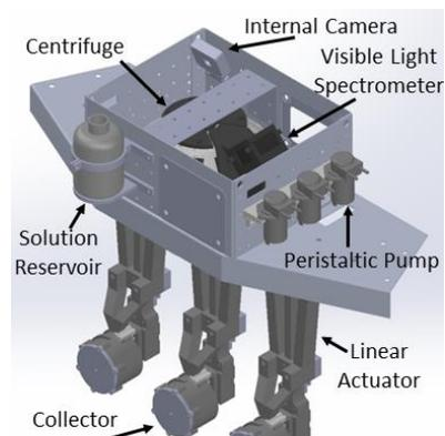
Figure 3: Annotated Drawing of science payload
